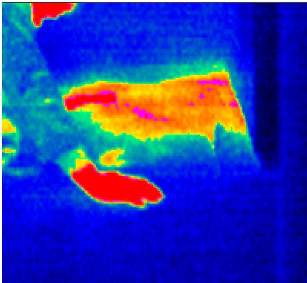
**Fig 3. Thermal image of a termite infestation in the floor of a house, near a corner in a room. Termite activity shows as red and yellow indicating a hot area. The hand and face of the inspector also appear red indicating heat of the body.**
