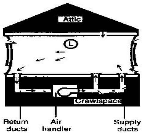
Figure 6. House depressurization due to supply duct leaks [1]
