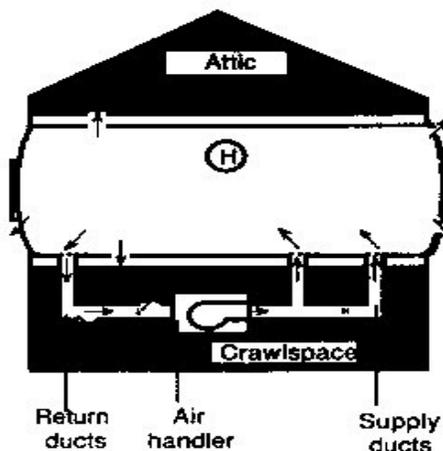
*Figure 11. Home pressurization due to return duct leaks [2]*
