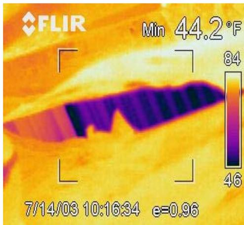
*Figure 10. Large leak in return plenum at air handler*
